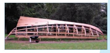
Hull on the strongback in Florida. Half of the first layer of planking is complete
