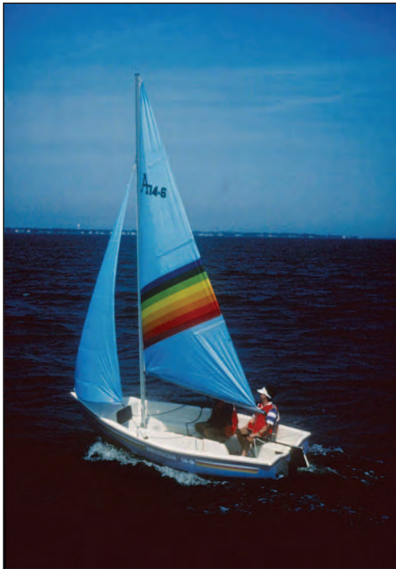
The A-14.6's wide beam and flat bottom give it excellent light-air performance and add stability.
