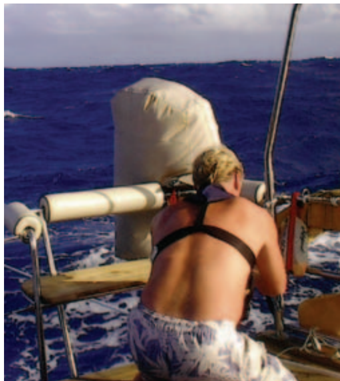
Joy For All crewmember David Grove fits an improvised chafe-guard, made from a leather deck shoe, on a storm drogue bridle.
