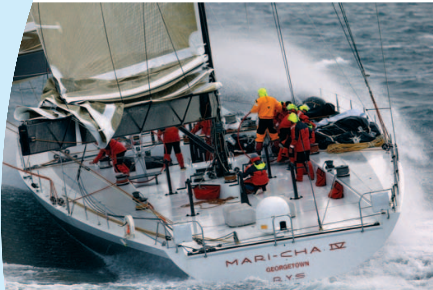
The 140-foot, carbon fiber Mari-Cha IV is capable of speeds of 36 to 40 knots.
