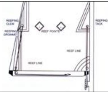
By using systems in place on your vessel, reefing of the sails is accomplished, leaving less sail area to catch the wind.
