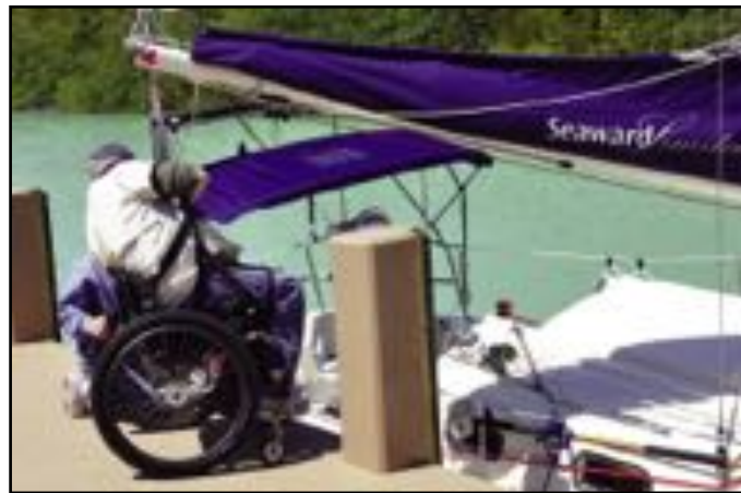
Kevin boards his specially outfitted Seaward 26RK with the boom hoist designed to lift him from the dock into the cockpit.
